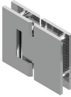
Adjustable 180° Glass-to-Glass Deluxe (80 lb./28" W max*) HI-DGTG180ADJ Self-Centering 0° Return with Adjustment Up to 30° In or Out Squared Edges Cutout Templates D
