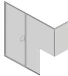
Semi-frameless w/ c-pull, panoramic center strike, aquarium corner, no threshold metal on notch rise, buttress, or return.
