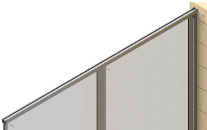
**Step 11:** Secure panel to header with thick push-in vinyl on both sides. Secure panel to bottom track with thin push-in vinyl on front side only.
