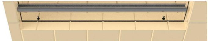
**Step 7:** Place the connected wall jamb and in-line snap post so that the bottom of the wall jamb sits in the base and the in-line snap post slides over the T-hold/panel. Plumb wall jamb with level and mark installation holes with felt tip marker. Drill holes using 3/16 bit and insert screw anchors. Secure with #8 x 1" installation screws. Secure panel with thin push-in vinyl on both sides.
