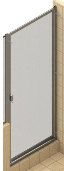
**Step 10:** Measure distance between walls across top of wall jambs and cut header at 1/16" less than opening. Slide over wall jambs and inline post. Drill holes at header through wall jambs and inline post. Secure with #6 x 3/8" screws.
