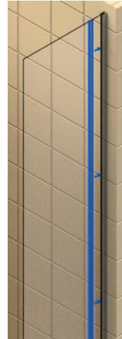
**Step 5:** Snap in-line snap post into wall jamb. Make sure that when the two pieces snap together that they are flush on top.
