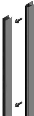
**Step 6:** Measure distance between wall and knee wall at base and cut bottom track at 1/16" less than opening. Place bottom track on base at center line.
