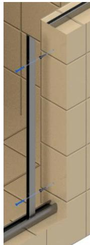
**Step 5:** Place wall jamb along back wall at center line so that it sits on the wall jamb that lies on the base. Plumb wall jamb with level and mark installation holes with felt tip marker. Drill holes using 3/16 bit and insert screw anchors. Secure with #8 x 1" installation screws.
