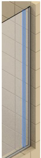
**Step 7:** Snap 90 degree snap post into wall jamb. Make sure that the tops of the two posts are flush with each other.
