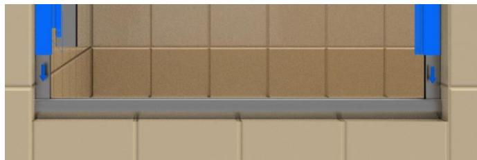
**Step 13:** Measure distance across top from outside corner of corner post to wall of front opening and cut front header 1/4" more than this dimension. Measure distance from outside corner of corner post to back wall and cut return header 1/4" more than this dimension.
