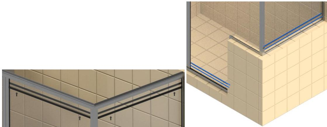
**Step 16:** Measure opening between hinge jamb and strike jamb. Cut threshold inserts to this dimension. Snap into bottom track and header.
