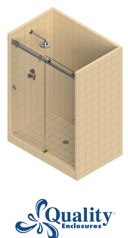
1) The Header Bar is positioned exactly in the middle of the two door panels. The Header Bar is generally mounted over the center of the threshold below. Note: Due to the extremely smooth nature of the Rollers, the Header Bar must be installed level. Failure to do so could result in sliding doors that roll to one side by themselves.
